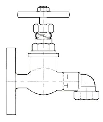
This fitting has Inspector's Test Gauge connection screwed 3/8" BSP female thread with a bronze elbow outlet.
