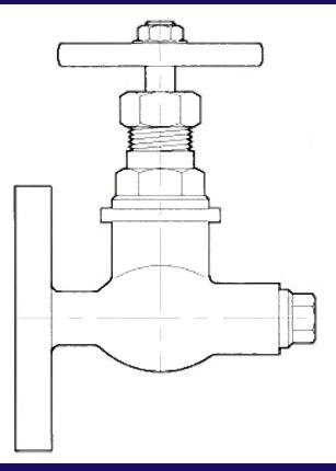
This fitting has Inspector's Test Gauge connection screwed %" BSP female thread and plugged.
